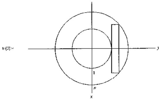
In the normalized representation,  $\vec{h}$  is a vector of magnitude  $n$  independent of free space wavelength. When the index is 1, the components are the direction cosines of  $\vec{k}$ .
