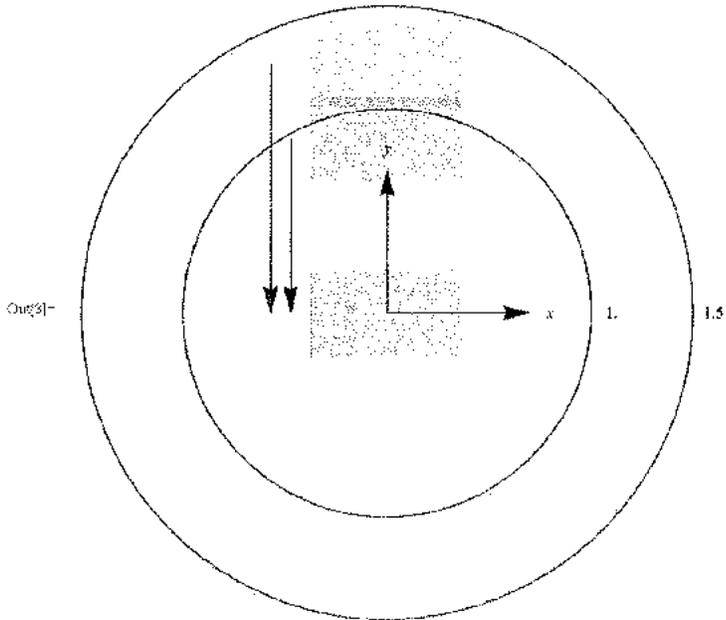
Tilting the substrate with respect to the eye is equivalent to biasing the eye field of view with respect to the substrate. This plot shows the effect of tilting the waveguide  $45^\circ$  and increasing the groove width to  $0.85 \mu\text{m}$ . Note that the
