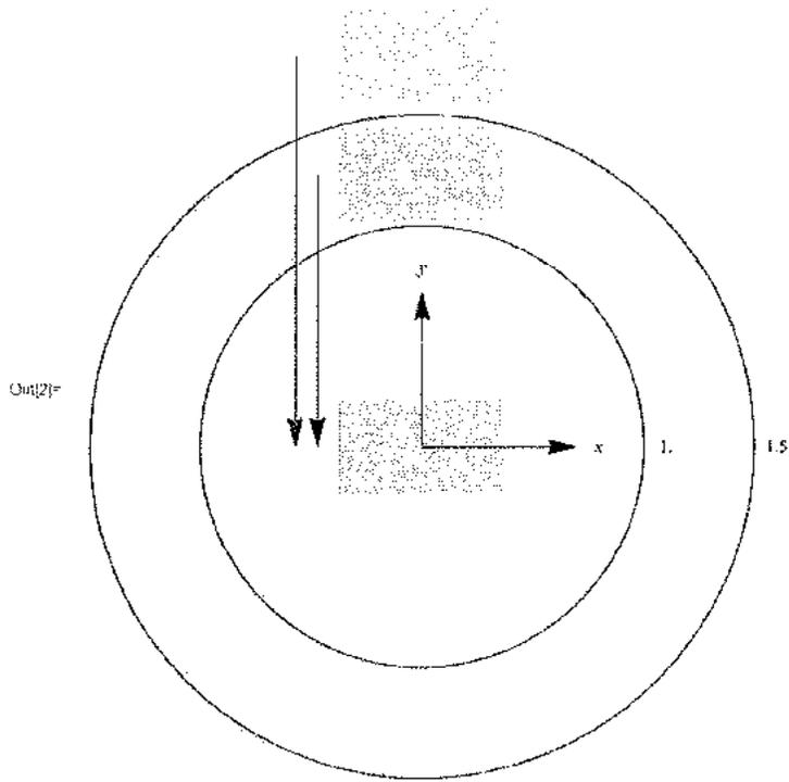
By increasing the groove spacing to  $5.2 \mu\text{m}$  the red wave vectors can be brought inside the allowed region, but then a majority of the blue wave vectors do not TIR.
